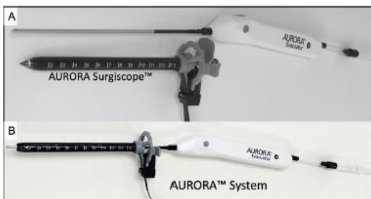
Figure 1 Aurora system consists of the Surgiscope and Evacuator (A), which is obtainable in 100 and 130 mm lengths. The Evacuator is connected to suction (controllable via the index finger) and contains a whisk to break up tough clot (controllable by the thumb). The whisk is rotated into the clot, away from brain tissue. The Surgiscope has a camera at the apex and LED lights at the tip, and is shown with the obturator in situ. The Evacuator is inserted into the Surgiscope (B) and protrudes distal to the tip for optimal clot engagement. Bleeding can be controlled by monopolar cautery applied to the shaft. Permission granted by Integra LifeSciences Corporation, Princeton, New Jersey, USA.
